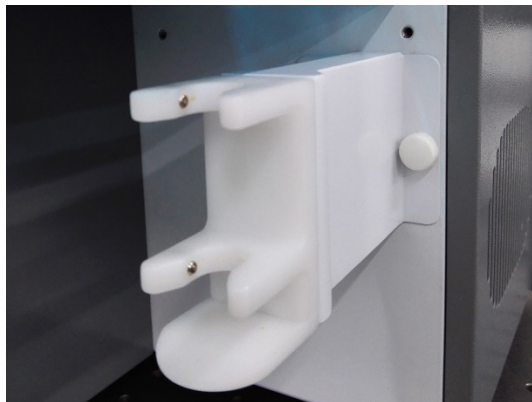
Figure 4. Remove the Tube Holder
