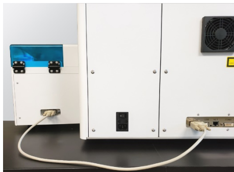
Figure 8. Connect NovoSampler Q to Agilent Flow Cytometer
